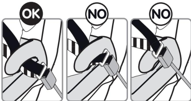
**EN** - In some cases, the strap attached to the seat belt buckle can be too long and ride too high under the armrest, preventing the car seat from being fixed firmly. If this happens, choose another location in the car. If you have any questions relating to this issue, you should contact the manufacturer.
