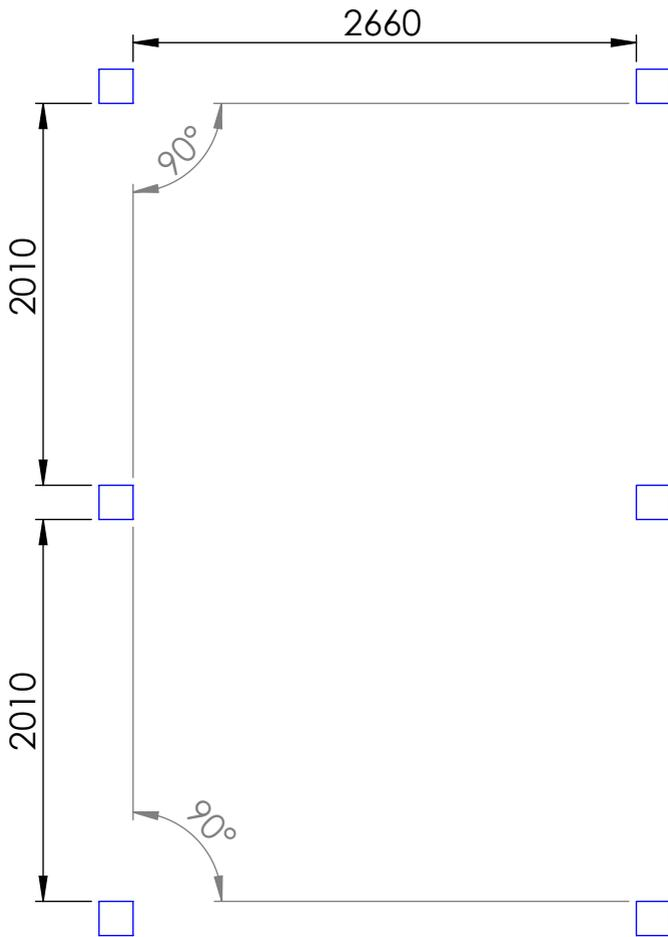
Plot Beton : 400x400x600mm
